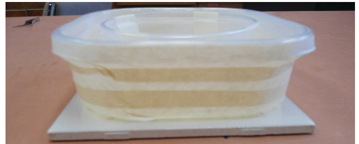
Figure 11. Square of tile placed underneath an interceptor trap.
