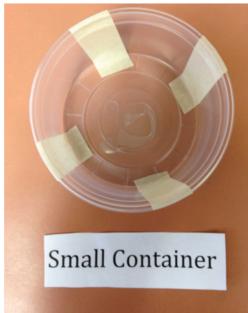
Figure 3. Rough-surfaced tape placed into the small container.
